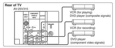
When you use VIDEO-1 INPUT, you should choose to connect S-VIDEO or video input. If S-VIDEO connector and video input are connected at the same time, no picture displays on the screen and the message "PLEASE DISCONNECT VIDEO-1 CABLE!" appears. In this case, you should disconnect either S-VIDEO or video input.
